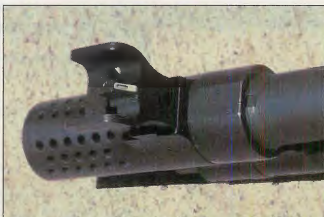
The XS 24-7 tritium-powered front sight comes standard on the SOCOM 16. The unique muzzle brake is integral with the gas cylinder lock and directs gas out top and side holes after pushing the muzzle forward.
